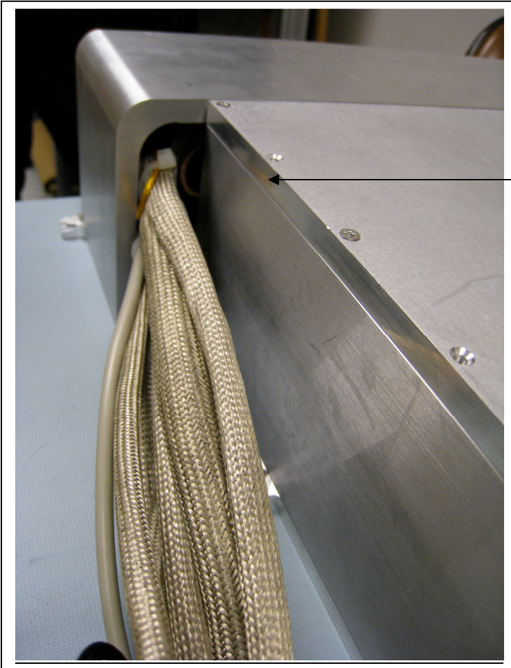
Harness Exit from IDPU Box (not installed: cable tie bases)
